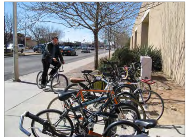
Bicycle rack designs should include racks that provide two points of contact with the bicycle so that it can be locked from both the front wheel/frame and the rear wheel.
