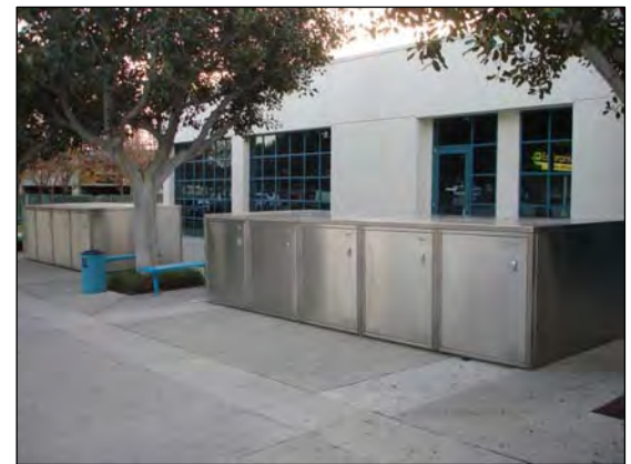
High-activity locations such as transit stations, offices, and major commercial districts should provide more secure, long-term bicycle parking options, such as bicycle lockers.
