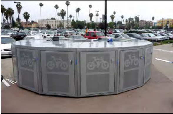
Bicycle lockers are appropriate end-of-trip facilities for civic activity centers and transit hubs.
