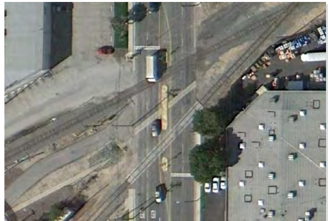
The angle of the existing at-grade railroad tracks is challenging for bicyclists to cross.
